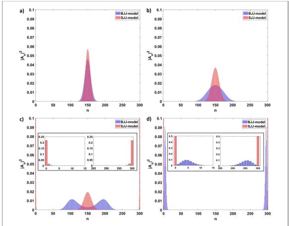
**Figure 3.** Ground state probabilities  $|A_n|^2$  vs n for (a)  $\Lambda=0$ ,  $\lambda=0$ ; (b)  $\Lambda=2$ ,  $\lambda=1$ ; (c)  $\Lambda\approx 2.000$  9925,  $\lambda=1.06$ ; (d)  $\Lambda=\lambda=4$ . The total particle number is N=300. Insets in (c) and (d) show the probabilities in the vicinity of 'edge' states with n=0 (left-hand panels) and N=300 (right-hand panels), respectively.
