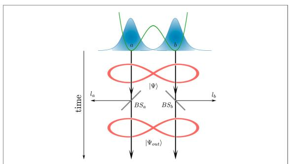
**Figure 6.** Scheme of particle losses from the condensate solitons trapped in double-well potential. Interaction with environment at each well are provided by means of fictitious BSs  $BS_a$  and  $BS_b$  in quantum channels 'a' and 'b', respectively.
