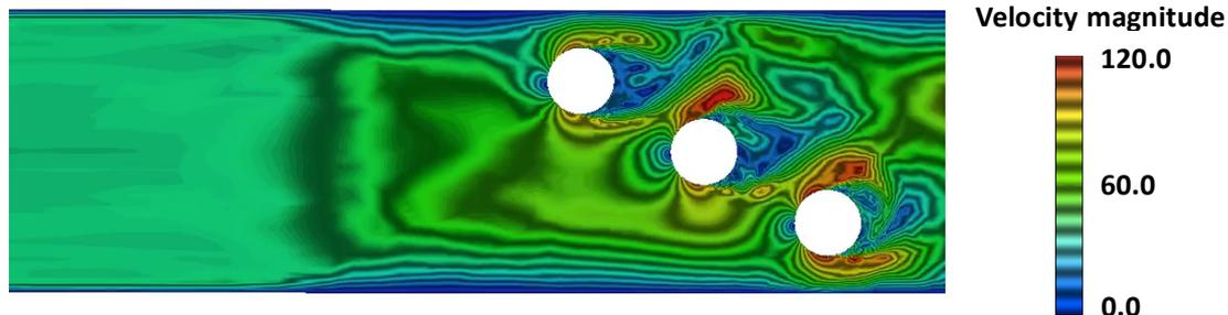
Figure 1. Cross-sectional view of the flow past three cylinders from 3D computation. The velocity magnitude is in m/s, and the cylinder diameter is 2 cm.
