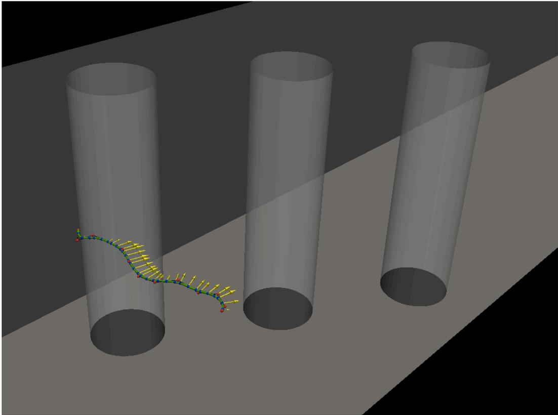
Figure 2. Cable dynamics when in contact with an obstacle. The arrows show the fluid force at each integration point along the cable.
