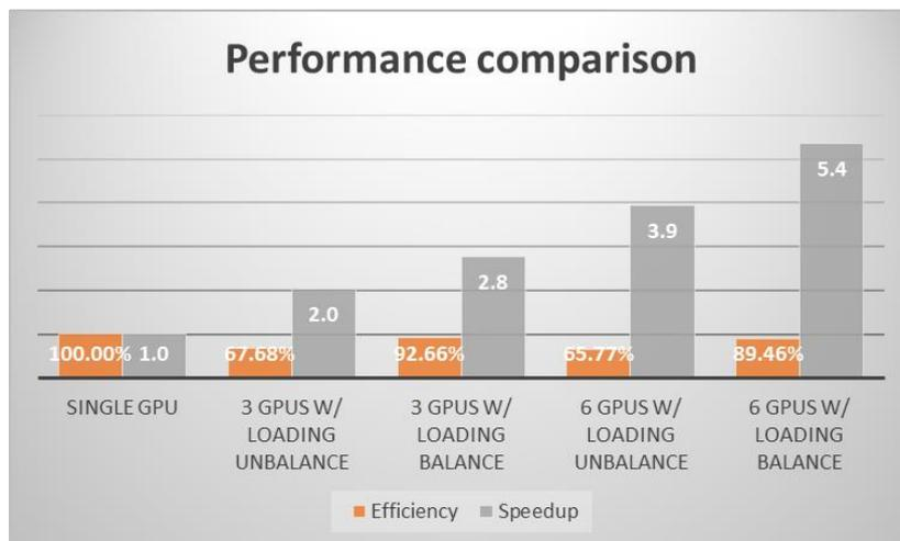
FIGURE 1 Comparison of those cases under the conditions including the different GPU numbers and loading balance method
