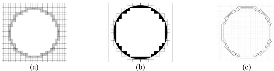
Fig. 1. (a) The shaded cells present a cylinder in a uniform Cartesian grid; (b) contour of the volume fraction function across the interface cells with subgrid; (c) contour of the volume fraction function across the interface cells without subgrid.
