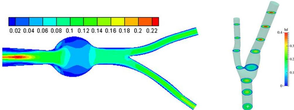
Fig. 2. Examples of 2D [8] and 3D [9] blood flow simulations using the GSM-CFD solver
