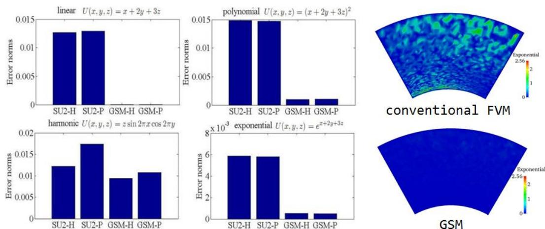
Fig. 1. Accuracy in gradient approximation of functions: comparisons with the most widely used FVM
