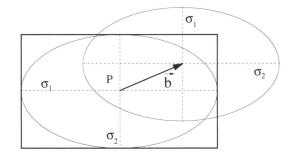
Figure 3: Principle of the BMO in two dimensions: The center of the mutation ellipsoid is shifted by the bias coefficient vector  $\vec{b}$  within the bounds of the step sizes  $\vec{\sigma}$ .
