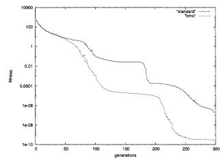
Figure 5: Fitness development of an (15,100)-ES with uncorrelated mutation with N steps sizes (standard) and with the BMO (bmo) on problem g04. On the y-axis the development of the difference between fitness and the optimum is shown on a logarithmic scale.
