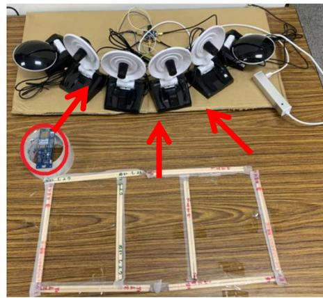
The photograph shows a hardware setup for CSI measurement. It features a multi-directional antenna array mounted on a wooden board, connected to a computer. A red circle highlights a specific component on the board.
