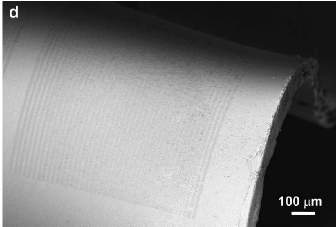
Figure 7. SEM images of the two-segment NW arrays a) on a ZnO substrate and b) after transferring on a flexible substrate. c) Bright-field optical image of the NW arrays on the flexible substrate. d) Low-magnification SEM image of the two-segment NW arrays on a flexible substrate. e) Current–voltage ( I – V ) curves of the as-transferred NW arrays in dark environment, under room light, and under UV illumination.
