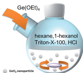
Fig. 1 The illustration of experimental design of GeO 2 nanoparticles synthesized in microemulsion system at room temperature.
