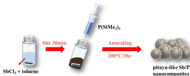
Figure 1. Schematic diagram of the synthesis of pitaya-like Sb/P nanocomposites.
