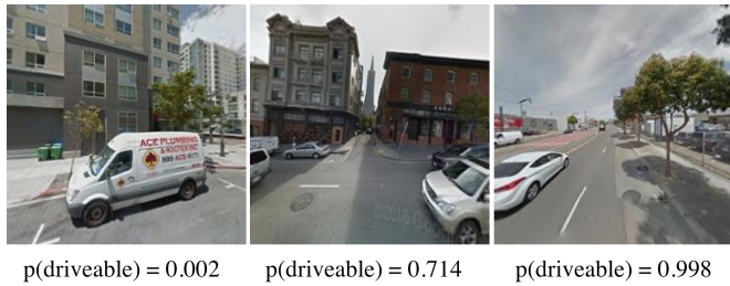
Fig. 6. Driveable headings. A ConvNet is trained to distinguish between non-driveable headings (left) and drivable headings aligned with the road (right). The ConvNet weakly classifies the middle example as drivable because the host car’s heading is facing the open alleyway between the buildings.
