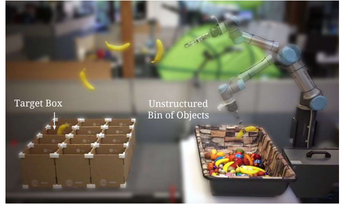
Fig. 1. TossingBot learns to grasp arbitrary objects from an unstructured bin and throw them into target boxes located outside its maximum kinematic reach range. The aerial trajectory of different objects are controlled by jointly optimizing grasping policies and predictions of throwing release velocities.
