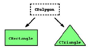
The class CPolygon would contain members that are common for both types of polygon. In our case: width and height. And CRectangle and CTriangle would be its derived classes, with specific features that are different from one type of polygon to the other.
