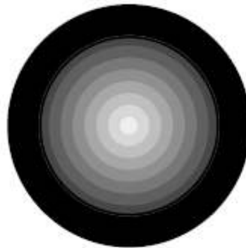
(b) The intensity in the fundamental mode LP_{01}
