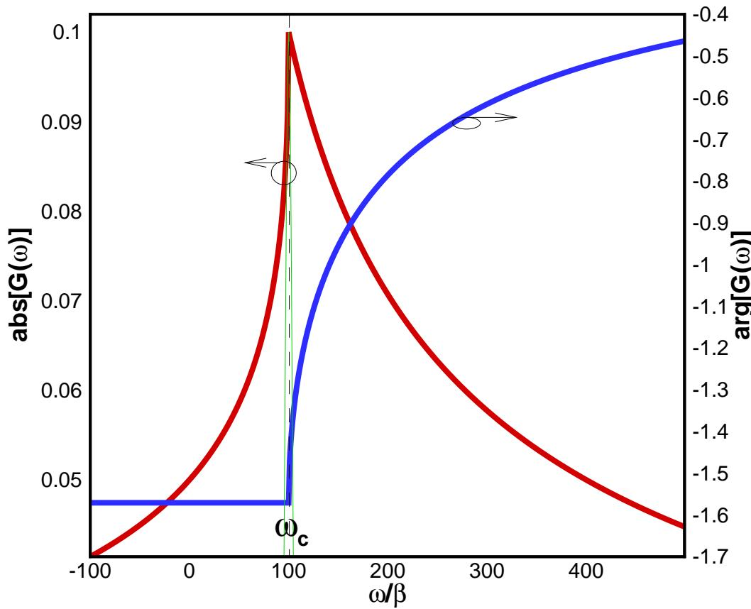
Amplitude and phase spectrum of the memory function
