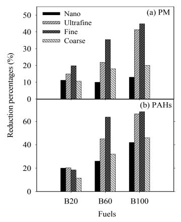
**Fig. 4.** Reduction percentages of (a) PM and (b) PAH emissions by biodiesel blending mixtures compared with D100.
