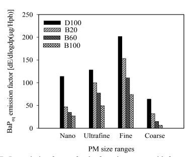
Fig. 5. BaP<sub>eq</sub> emission factors for the four size ranges with four test fuels.
