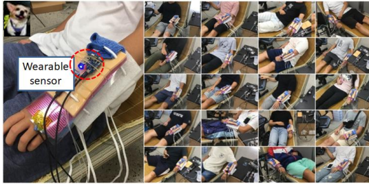
Fig. 14. The artificial skin installed on the arm of participants during the experiments
