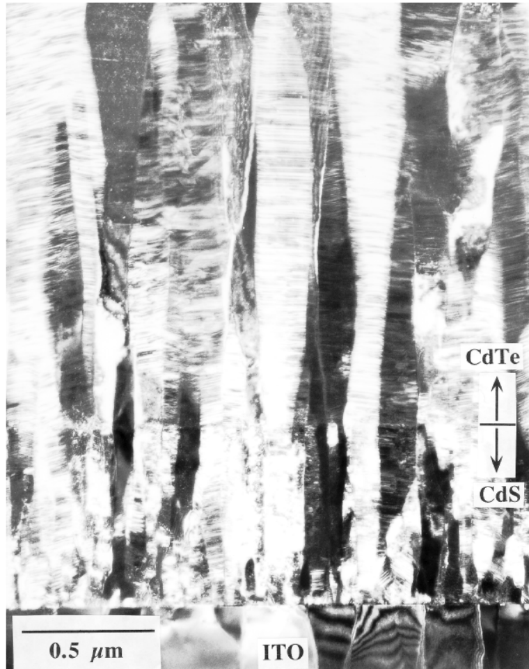
Figure 9 TEM micrograph showing the as deposited cross section of ITO/CdS/CdTe structure. Both CdS and CdTe are vapor deposited from the respective compounds.
