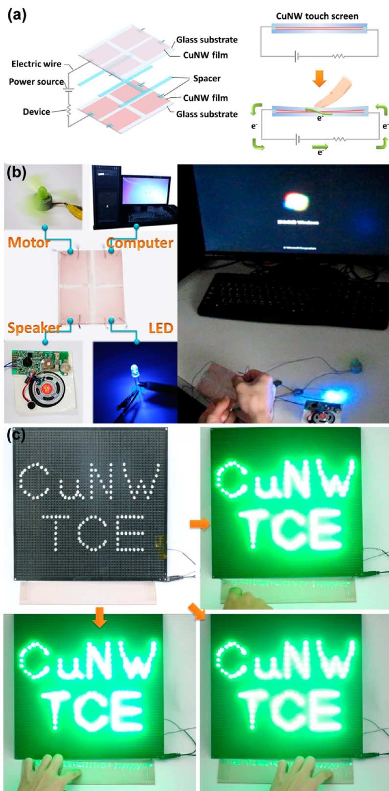
Figure 8. (a) Schematic diagram of the structure of CuNW touch screen (left) and concept of CuNW touch screen (right). (b) The 6.5 × 10 cm 2 CuNW touch screen fabricated by two CuNW TCEs was applied in turning on the computer, LED, electric fan, and speaker. The associated video showing the operation details is shown in video S1 . (c) The 6 × 25 cm 2 CuNW touch screen was applied in lighting a LED array, circuit is form by touching different places on the touch screen. The associated video showing the operation details is shown in video S2 .
