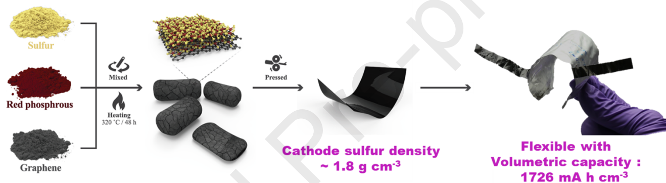
Scheme 1. Schematic diagram of the process for fabricating PS/G composites materials.
