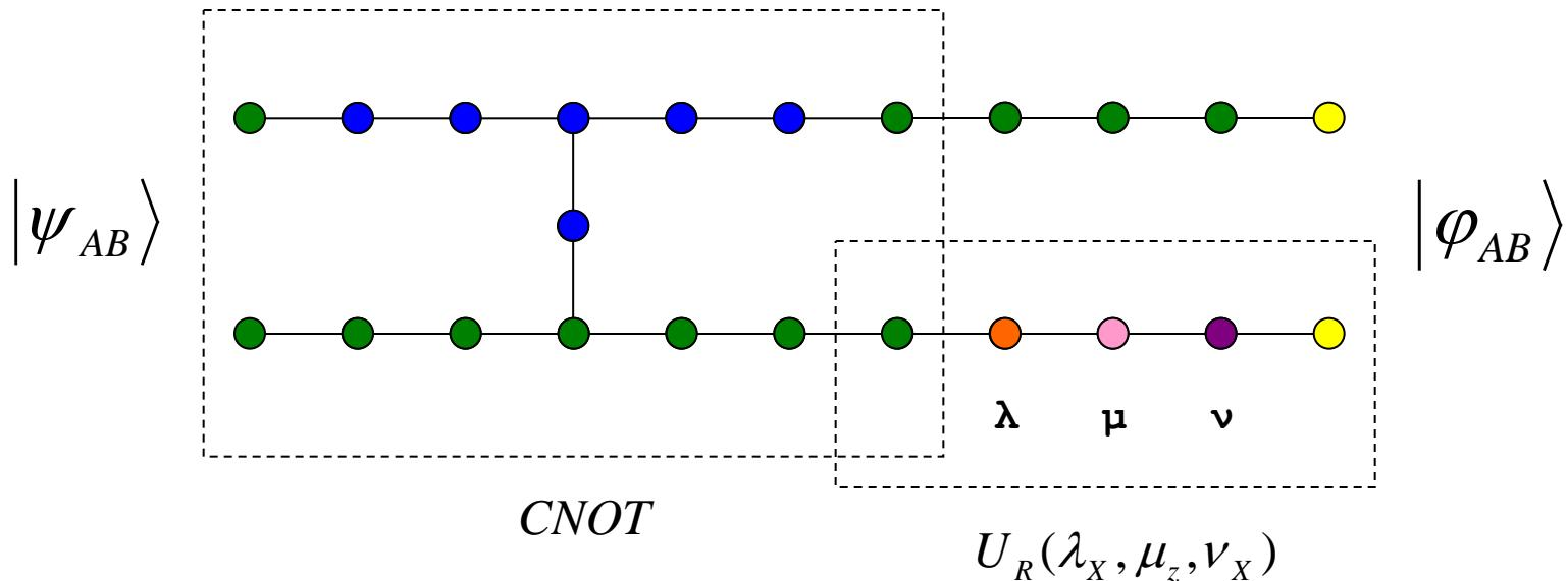
$$|\psi_{AB}\rangle \mapsto |\varphi_{AB}\rangle = U_{\Sigma} U_R^{(B)} CNOT^{(A,B)} |\psi_{AB}\rangle$$
