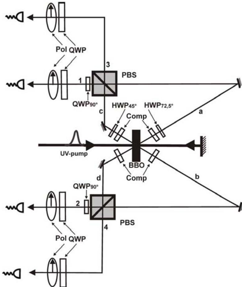
UV laser pulse (395 nm) makes 2 passes through BBO crystal to produce (including double pairs)
